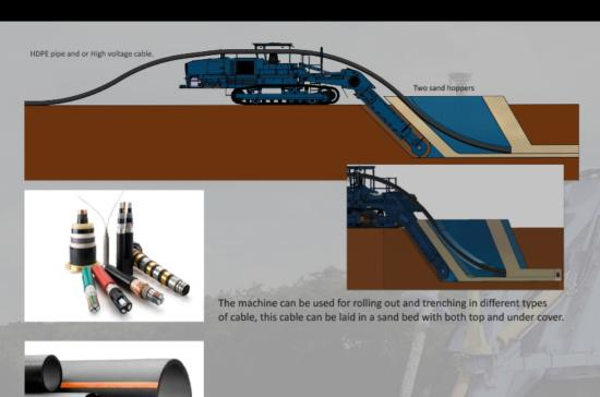
The machine can also be used to trenching different diameter pipes, this varies up to 800 mm with a minimal disturbance of the soil structure. Other diameters and specials on demand.
